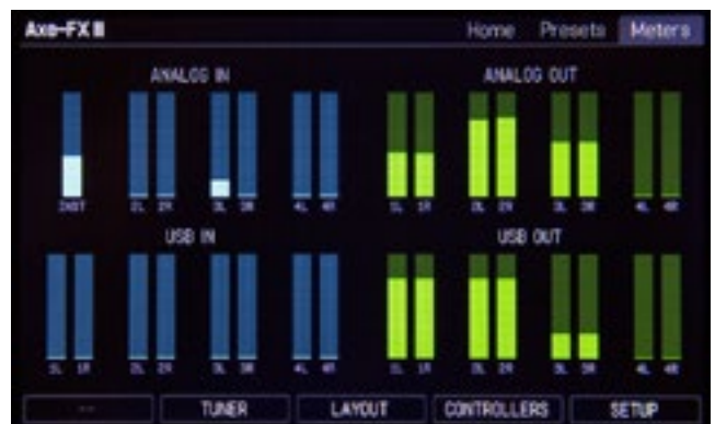
The Meters page of the Home menu shows all I/O levels.
